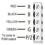
① **Note:** When using end of line supervision, connect the zone according to one of the configurations outlined in Zone Wiring. End of line resistors must be placed on the device end of the loop, not at the keypad.
