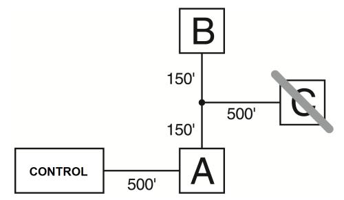
Module (A) is wired correctly as it is within 1,000'/305m of the panel, in wire distance. Module (B) is wired correctly as it is within 1,000'/305m of the panel, in wire distance. Module (C) is NOT wired correctly as it is farther than 1,000'/305m from the panel.
