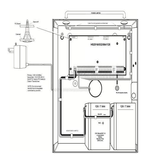
Figure 2: Wiring Routing (EN50131 only)
