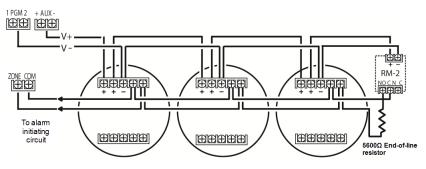
Figure 15: Smoke Detector Wiring
